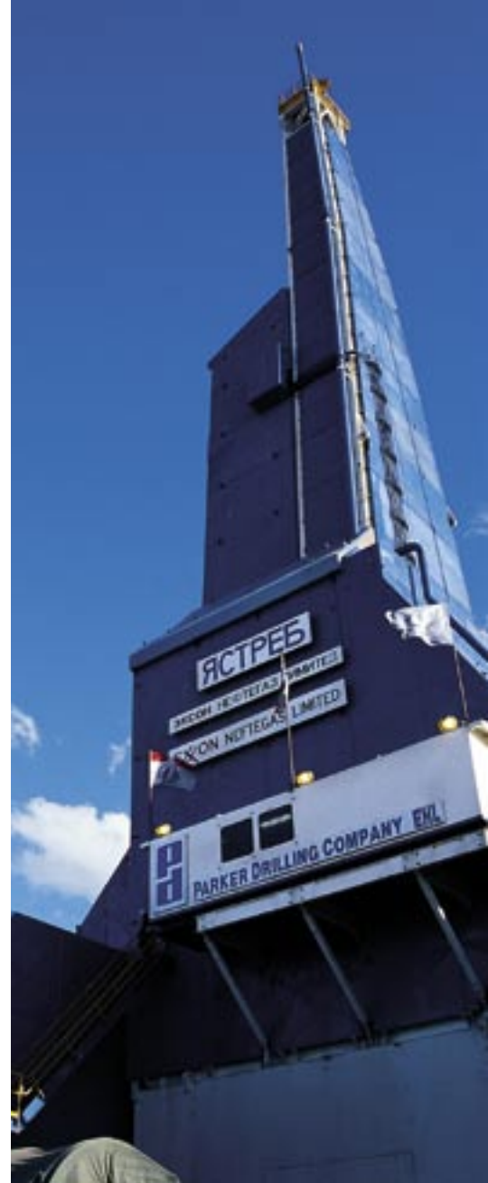
The 22-story Yastreb rig will drill more than 20 extended-reach wells, including some of the world’s longest.
