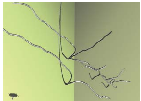
Actual multilateral, fishbone well trajectories targeting shallow reservoirs from a single mother bore. (Image courtesy of Schlumberger)
