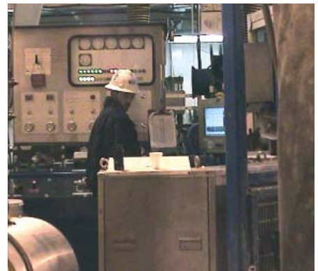
A Parker Drilling crew member shown while drilling the first Sakhalin-1 extended-reach well. Data on current activities and drilling progress is transmitted to the driller on the floor, rig offices and the drilling contractor's headquarters. Drilling engineers on-site and remotely can analyze drilling performance in real time. In addition to drilling performance, equipment packages such as the top drive and diesel engines transmit real-time performance information to remote locations. Maintenance issues can be evaluated and recommendations made by technicians working off-site. (Photo courtesy of Parker Drilling Company)
