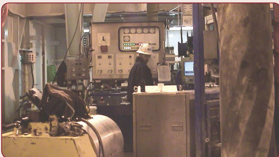
Drillers use the Yastreb's cutting-edge technology to steer the bit and measure progress while drilling. The data are transmitted to the driller on the floor, rig offices and Parker Drilling's Houston office. Drilling engineers on site and remotely can view the data and analyze drilling performance in real time.
